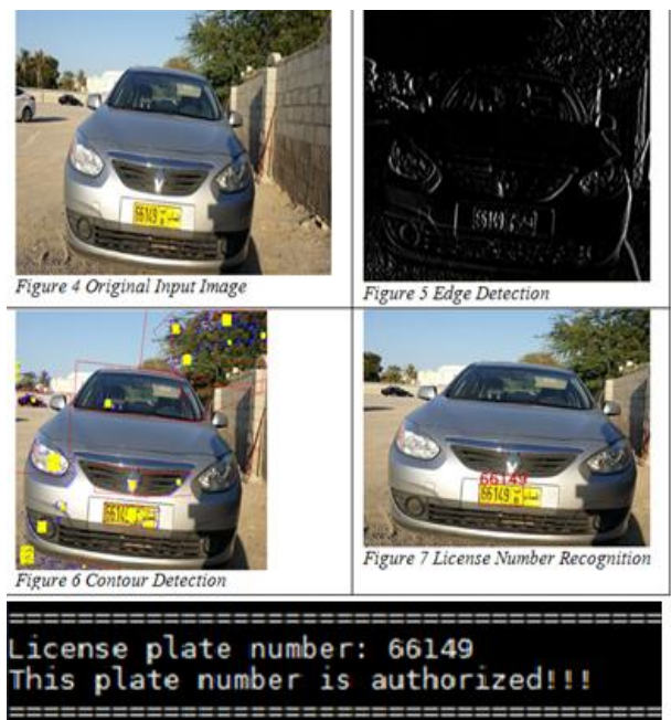
Fig 4: Example of Number Plate Recognition
